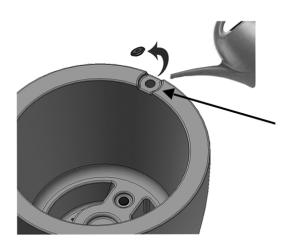
Remove fill port plug for direct access to the water reservoir.
